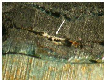
*Grayish-white deposit with some streaks of red, typical of acid phosphate deposits.*
