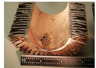
**Close-up of the ID deposit and pit. 1.2x -This is a HRSG Heat Recovery Steam generator tube example.**
